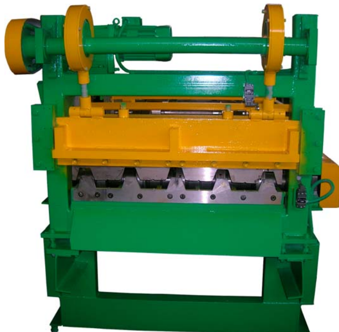
Guillotine-type electromechanical shears
